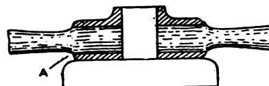
Thin Wedges, Placed Under Opposite Sides of the Hub Flange on a Wheel, Straighten the Rim
